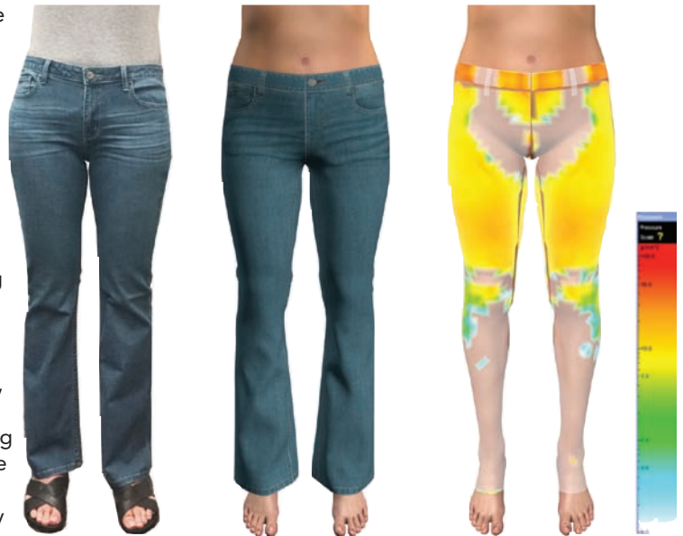
The same pair of jeans is shown on a physical model (left) and 3D virtual model (center). Then at right is a view of 3D pressure mapping of how tightly or loosely the garment fits. VF Jeanswear teams use this information for making changes and interpreting consumer fit feedback. Image courtesy of VF Jeanswear.
